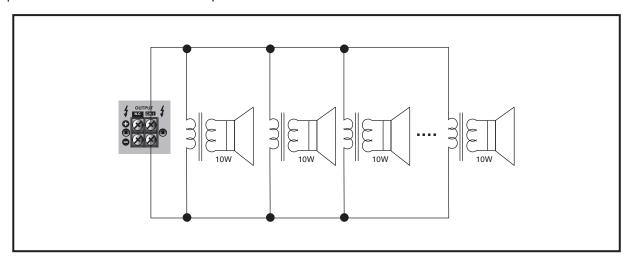
**Caution:** 1. Make sure that the total impedance does not equal or less than the rated impedance.
